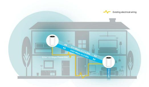
Deco PX50 = Dual-Band Wi-Fi 6 + G.hn Powerline + Seamless Al-Driven Mesh + HomeShield
